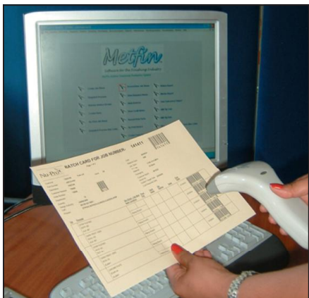
'Metfin' is bar-code enabled – any manual entry can be by bar code, including raising delivery notes and job tracking.
